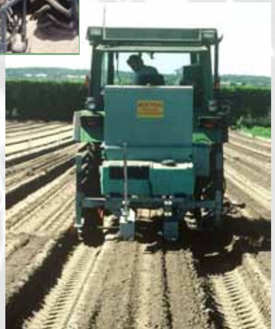
Demonstration models showing application of granules or liquids to soil with modified equipment.
