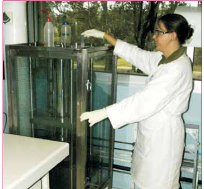
Tanya James, Technical Officer Scientific, prepares to test thrips for insecticide resistance with the aid of a Potter precision spray tower.
