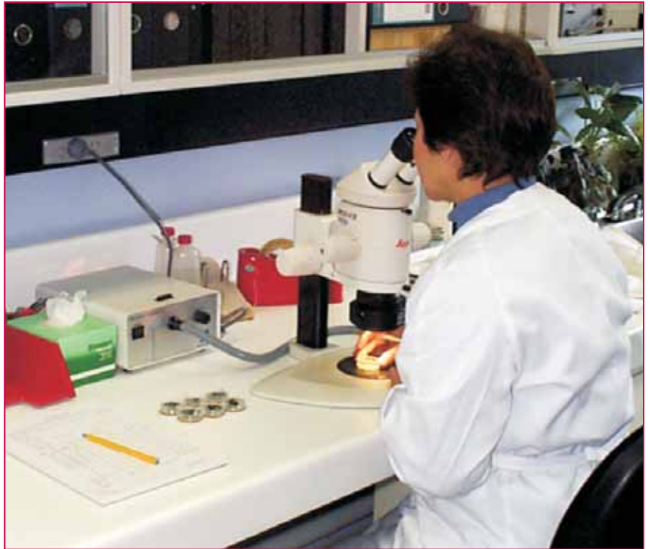
Jeanette Rophail, Senior Technical Officer, scores a resistance test under a stereo microscope.
